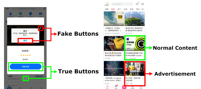
(a) An example of fake button which triggers user unwanted behaviors. (b) Disguised Advertisement whose layout is similar to normal in-app content.
